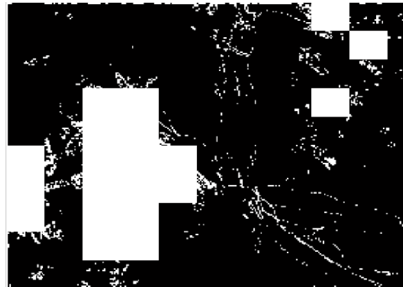
Fig 8: Final output after filtering showing the weed affected areas as white blocks.
